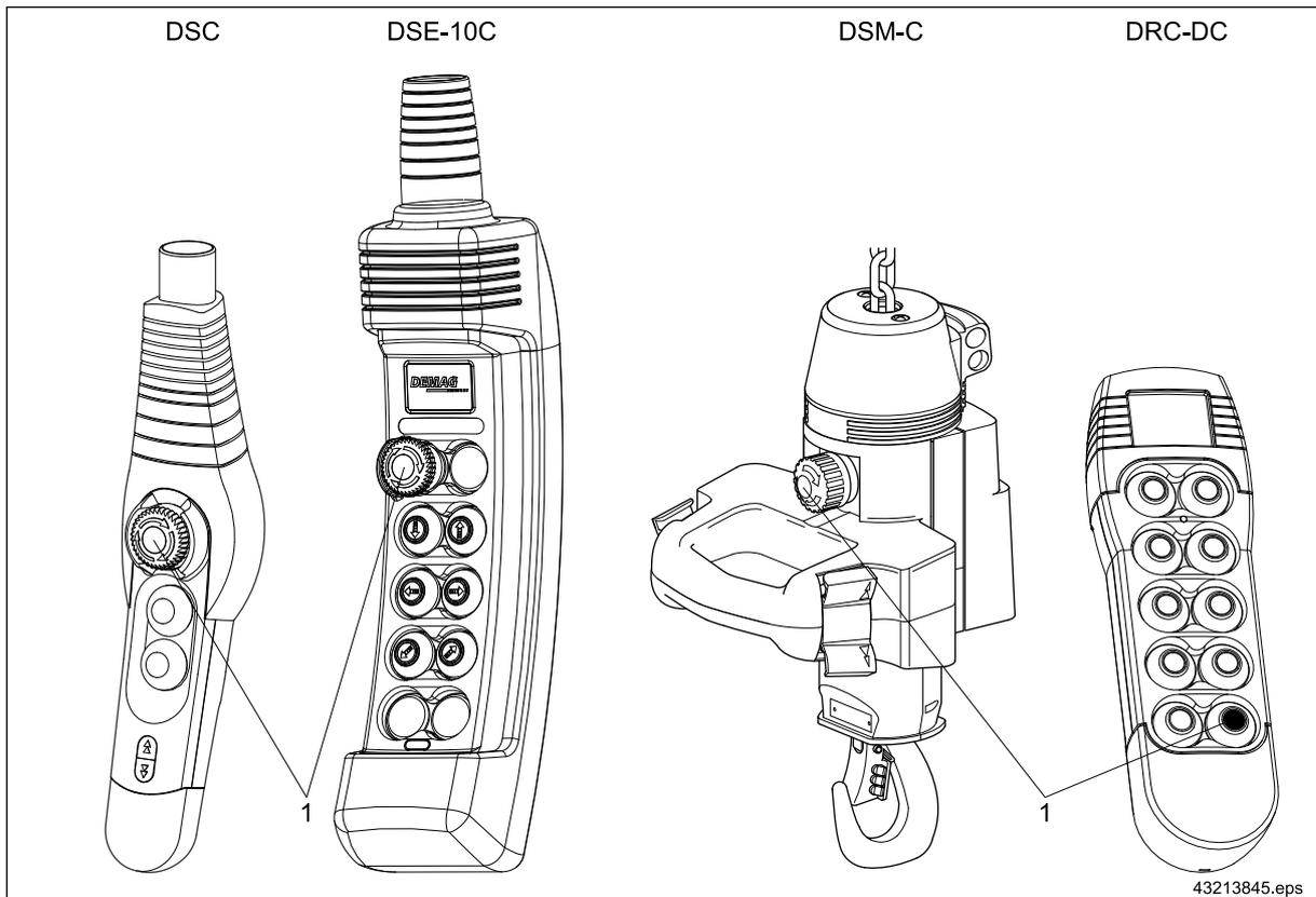
Fig. 38 Position of the emergency stop (1), DC-Com not connected to DSM-C
