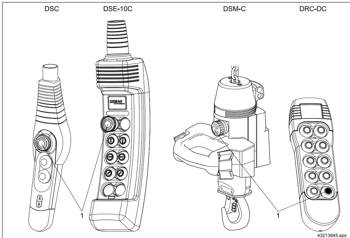
Fig. 3 Position of the emergency stop device (1)
