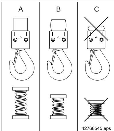
Fig. 44 Buffer with **limit switch not being actuated** (A), buffer with **limit switch being actuated** (B), **defective buffer** limit switch being actuated (C).
