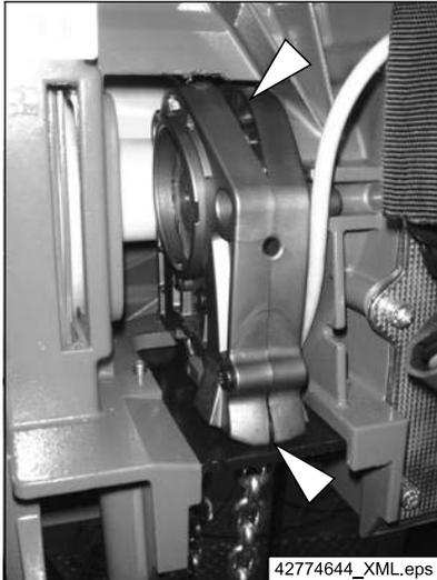
Fig. 45 Example for defective chain guide
